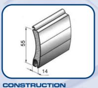
The 55 x 14mm profile of the €uropa Compact is the industries leading product in insulation and sound reduction. Its slimmer design allows it to coil tighter, therefor requiring smaller head plates than that of the €uropa. The strength of the profile has also been vigorously tested, and spans openings of up to 3000mm.
